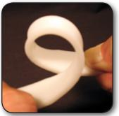
Advanced Laser Materials' RM<sup>2</sup> 250-C is a specially formulated polyamide engineered for laser sintering. The exceptional breakthrough in the RM<sup>2</sup> 250-C material is its high process stability. The polyamide bases of the RM<sup>2</sup> 250-C are engineered to ensure that un-sintered powder can be repeatedly reused in your production process. This means little to no waste product from your process and a considerable material cost savings.
